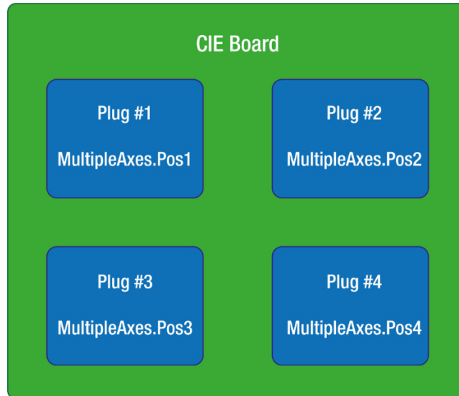
Example of configuration compatible with multi-axis PSO
